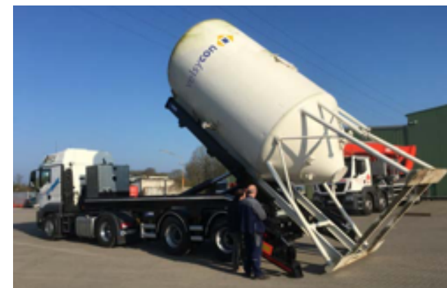
Taking up silos according to DIN 30734 at the lateral acceptance hinge.
